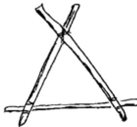
Square shapes or trestles must be strengthened with diagonal braces to keep them square. Lash all of the poles that make up the square first. When the square is completed, lash the two diagonal poles by attaching the lower lashings before the upper lashings. When the upper lashings are done, make sure that the structure is square. All of the lashings are Square Lashings. The top of the trestle is always smaller than the bottom.
